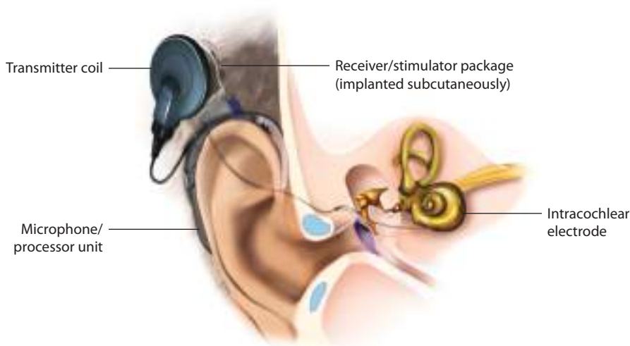
Figure 55.1 Basic structure of device. The microphone/processor/battery pack and transmitter coil are worn externally while the receiver/stimulator package and intracochlear and electrode lead are surgically implanted. (Courtesy of MED-EL.)
